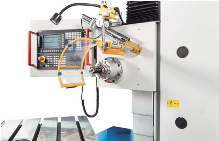
Milling spindle cover with safety switch
