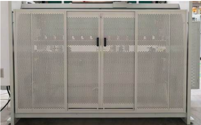
Rear Safety Doors Equipped with a safety interlock system, the rear door prevents access while the machine is in operation, ensuring maximum protection. The safety switch automatically cuts power when the rear door is opened, reducing the risk of accidents during service.
