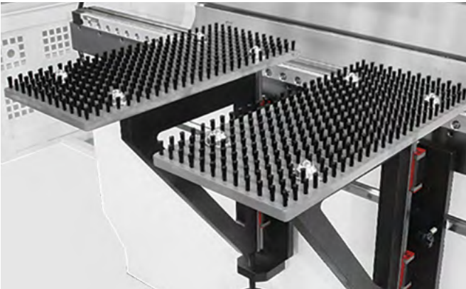
Brush Front Support (optional) Brushed front support minimizes surface damage on the sheet, ensuring clean processing and reliable positioning throughout the operation.
