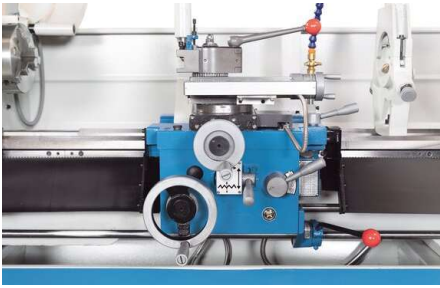
Support with enclosed oil-bath for low maintenance
