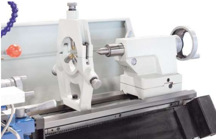
Rigid rests significantly increase turning precision and efficiency
