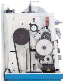
Change gears provide for a wide range of thread leads and feeds
